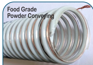
Temp. : 80°C Wall Thick. 0.75 to 1 mm PU Hose With Rigid Helix (Antistatic Copper Wire)
