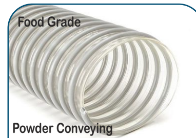
Food Grade Powder Conveying Temp. : 80°C Wall Thick. 0.75 to 1 mm PU Hose With Rigid Helix (Antistatic Copper Wire)
