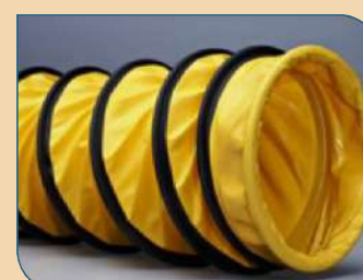
POLYESTER FABRIC HOSE PVC COATED Flame Retardant / Outer Wearstrip Profile Range: 150 mm to 3500 mm Temp. -20°C to 80°C
