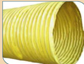
POLYESTER FABRIC HOSE PVC COATED - UV RESISTANT Heavy Duty - Flame Retardant Range: 38 mm to 1000 mm Wall Thick.: 0.5 mm Temp. -20°C to 70°C
