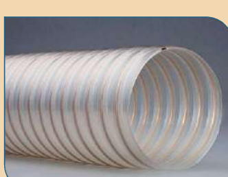
FLEXADUX HT PU POLYURETHANE HOSE FOR HIGH TEMPERATURE APPLICATIONS Wall Thick. 0.7/1/1.4 mm Temp. -40°C to +145°C (Short-term: +165°C)
