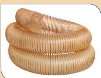
PU HOSE - HEAVY DUTY Ether Grade Wall Thick. 0.6 / 0.7 / 1 / 1.2 mm Temp. -40°C to +100°C (Short-term: +125°C)
