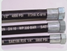
B.P : 163 to 920 kg/cm 2 W.P : 40 to 230 kg/cm 2 Temp : 40°C up to +100°C HYDRAULIC HOSES
