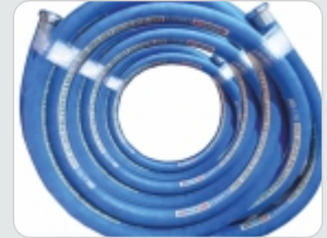
W.P : 16 kg/cm 2 Steam Cleaning up to +130°C (for Max 30 Minutes) B.P : 48 kg/cm 2 Temp : -25°C up to +100°C FDA-GRADE CHEMICAL HOSE - UHMWPE
