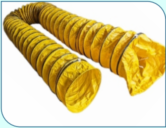
HVAC - Ventilation Hose Yellow Fabric Hose UV / Flame Resistant Range: 38 mm to 609 mm Wall Thick. 0.5 mm Temp. -20°C to +70°C
