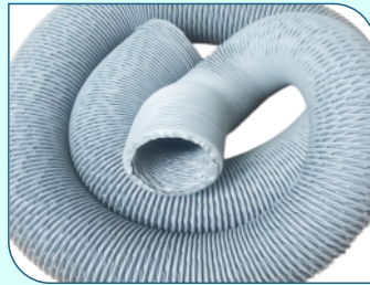
POLYESTER FABRIC HOSE PVC COATED UV Resistant and Fire Retardant GREY - LIGHT Range: 50 mm to 600 mm Wall Thick.: 0.25 / 0.3 Temp. -20°C to 70°C
