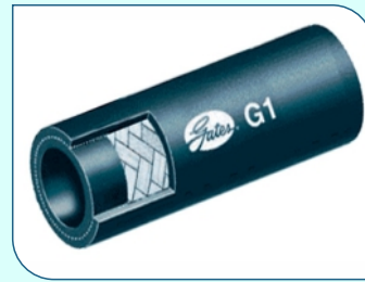
HYDRAULIC HOSES SAE R1 AT Range : 6.3 mm to 50.8 mm W.P. 40 to 230 kg/cm 2 B.P. 163 to 920 kg/cm 2 Temp. -40°C to +100°C
