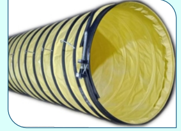
POLYESTER FABRIC HOSE PVC COATED Fire Retardant / Outer Wearstrip Profile Range: 150 mm to 3500 mm Temp. -20°C to 80°C
