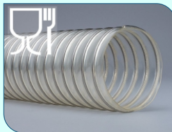
PU HOSE FDA APPROVED FLEXADUX P7 L & M PU PAS FOOD FOOD GRADE - FDA APPROVED PERMANENTLY ANTISTATIC WITH SS 304 WIRE Wall Thick . 0.7/ 1.4 mm Temp. -40°C to +100°C (Short-term: +125°C) ( PAS FOOD )
