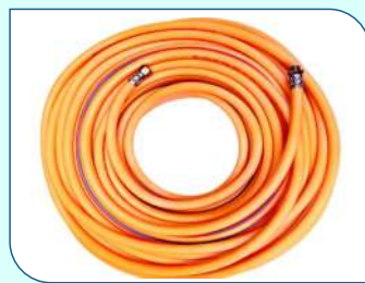
HIGH PRESSURE AIR CLEANING HOSE Range : 8.5 mm to 20 mm W.P. 30 to 60 kg/cm 2 B.P. 120 to 225 kg/cm 2
